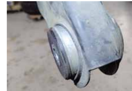
AND THIS LOWER WAS SO BAD IT WAS RATTLING AROUND...SO IT GOT ONE NEW ARM THIS TIME
