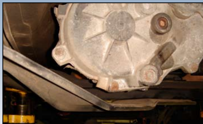
Transfer case is now clearing the bash plate with the new mount fitted
