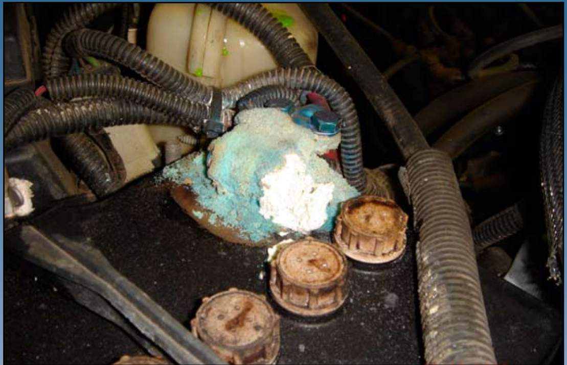
Badly corroded battery terminal
