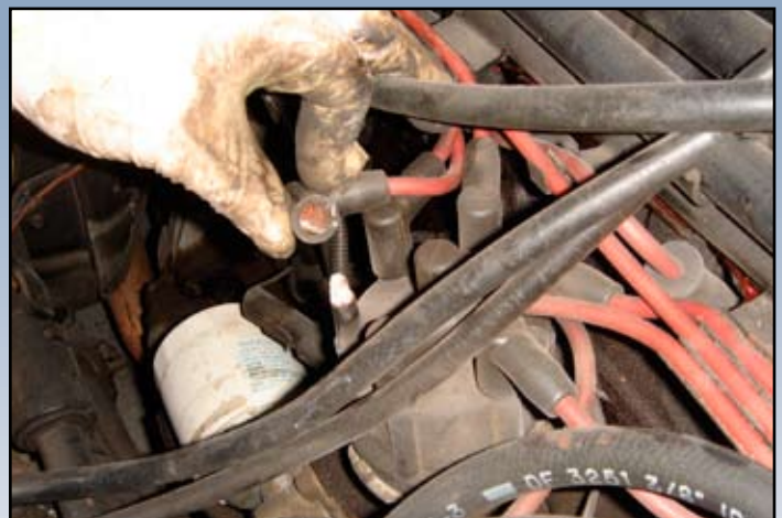
Corroded distributor cap post
