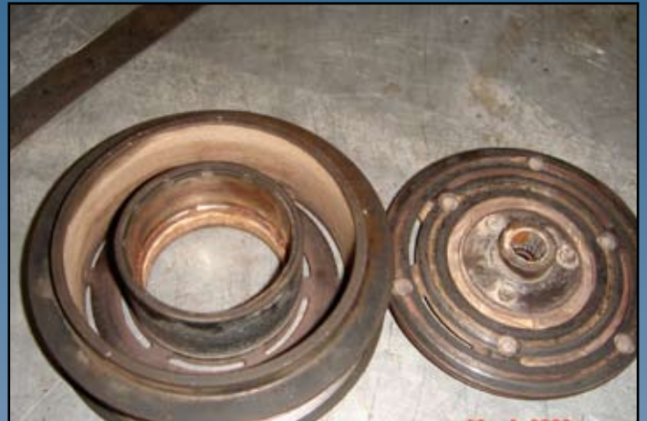
Clutch face assembly
