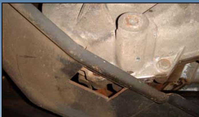
Hole cut in transfer case bash plate
