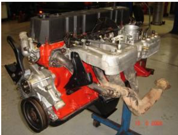
water pump, EFI manifold and extractors fitted
