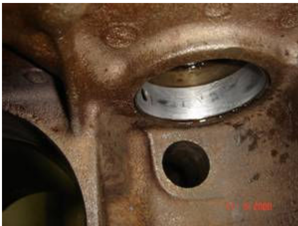
A badly worn cam bearing, the soft alloy have worn away
