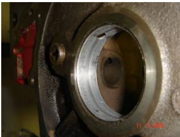
The rear main cap bearing was good to reuse a decent cam bearing
