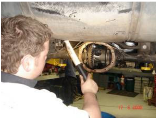
Nick checks the D35C LSD, it had been run dry!
