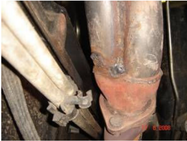
The Patched up 4.0 manifolds are common place.
