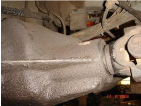
Tell tale diff issue with massive pinion leak
