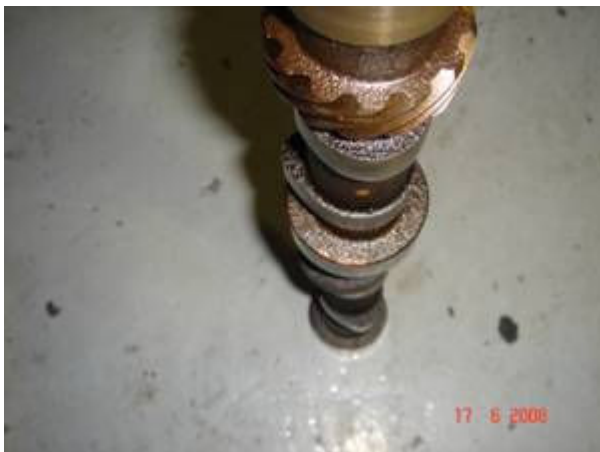
The cam lobe below the distributor drive is rounded
