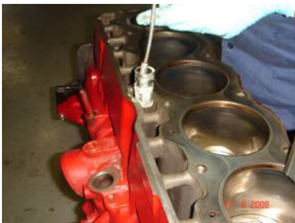
Lifters come out the same way the new ones go in.
