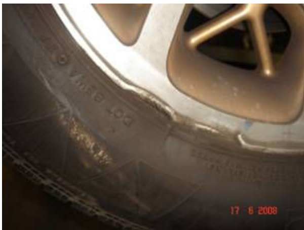
Rim damage to the front right wheel.
