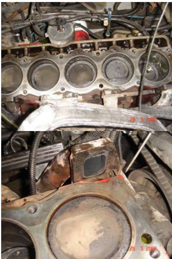
The motor before removal to add to the fun there was a snapped head stud
