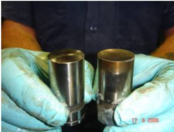
The new lifter on the left, the worn lifter on the right
