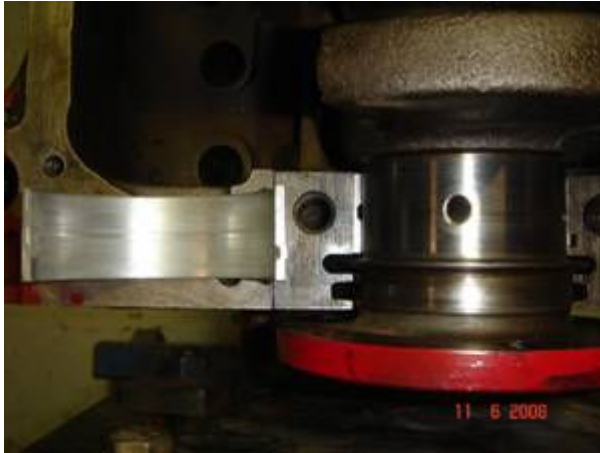
The rear main cap bearing was good to reuse a decent cam bearing
