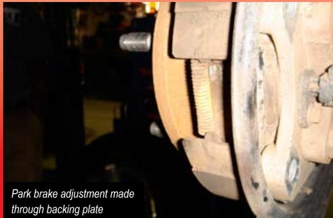
Park brake adjustment made through backing plate
