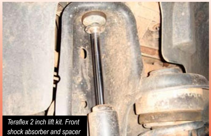
Teraflex 2 inch lift kit. Front shock absorber and spacer
