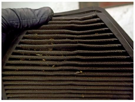
hose, they come up like new before your eyes, then shake it dry, don't use compressed air as it can tear the cotton filament, then sit it in the sun to dry before re-oiling it. And don't over oil it either, too much oil will block air flow and in some machines with carbies they will run rich with fuel and run like a dog.
