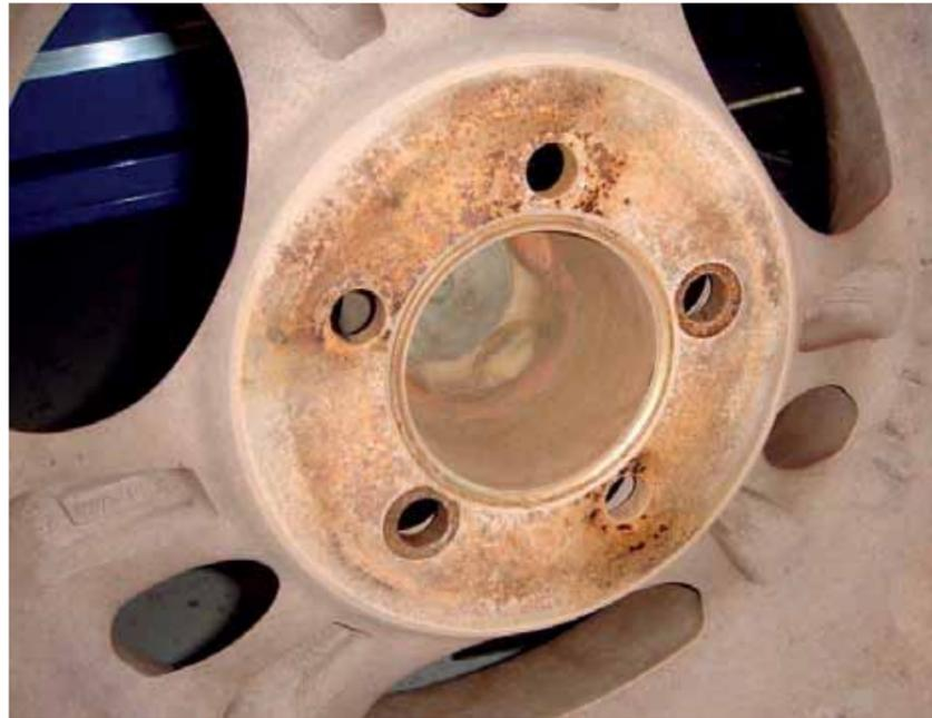
a wheel that's not sitting flat on the face surface and in some cases can wobble loose and snap studs. We get calls all the time for replacement studs exactly from
