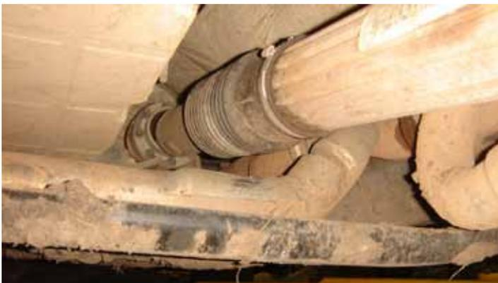
After removing the over kill shock brackets all there was left on the front cross over pipe was a mark and a worn drive shaft boot. These boots are still impossible to source on their own.
