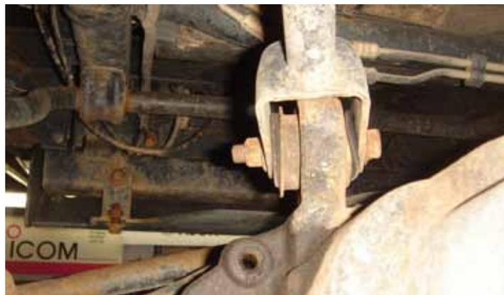
*The bent rear panhard and no front panhard was contorting it's control arm bushes badly at full droop. It's so important to do every aspect of a lift kit to get it right and make it last. If you lift it you need to bump stop it, extend sway bar links, brake lines, drop or lengthen panhard rods and set up caster angles. These bushes will be dead soon and this Jeep has only 24K on the clock.*
