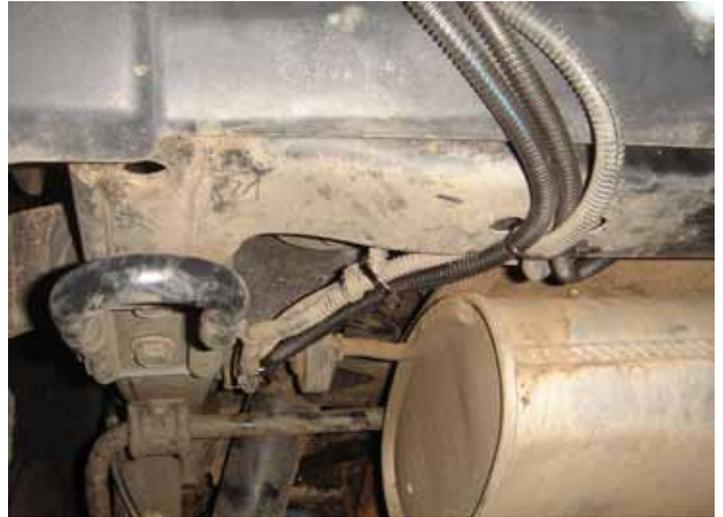
The "auto electrician" had run all the trailer loom under the cross member, the thing you slam on the ground, bump off and jack up from. We had to refit the lot to hide it and protect it from damage, this is simple stuff that should be done right first time.
