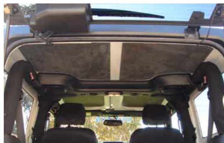
Panel set installed in the 2012 JK 2 door.
