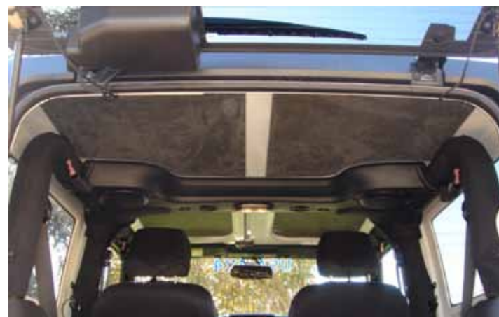
Panel set installed in the 2012 JK 2 door.
