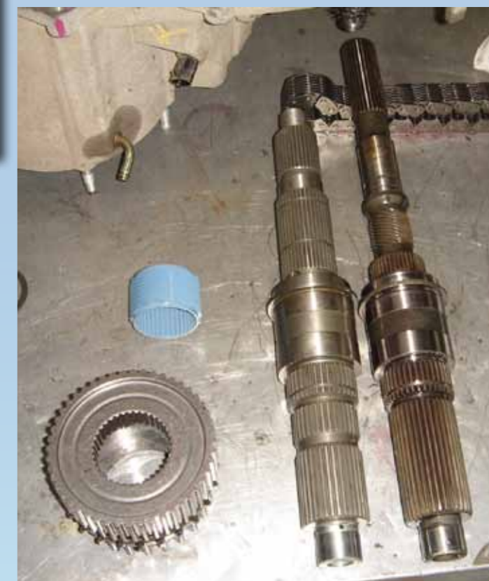
The blue spiral collar is the new drive compared to the steel spiral on the right.
