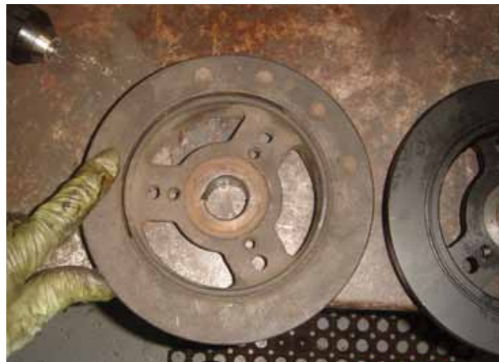
Here is the old balancer missing sections of rubber and the new one on the right ready to go on.
