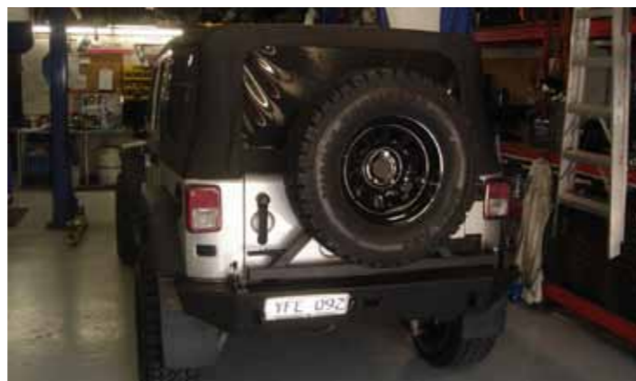
The matching rear WARN bar and tyre mount
