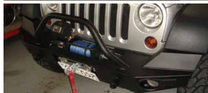
A close up of the WARN elite bar and VRS 9500 plasma rope set up
