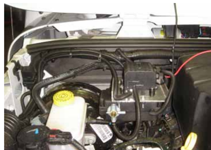
JK my ride pump install. There isn't a lot of space under the JK hood, especially the 2012 model, to fit the My-ride pump and controller. We utilized the fire wall bracket on the driver side and wired into the fuse box. you have to have a switch able power source for the My-ride as they can ghost operate when not required if hard wired when they sense a drop in line pressures.
