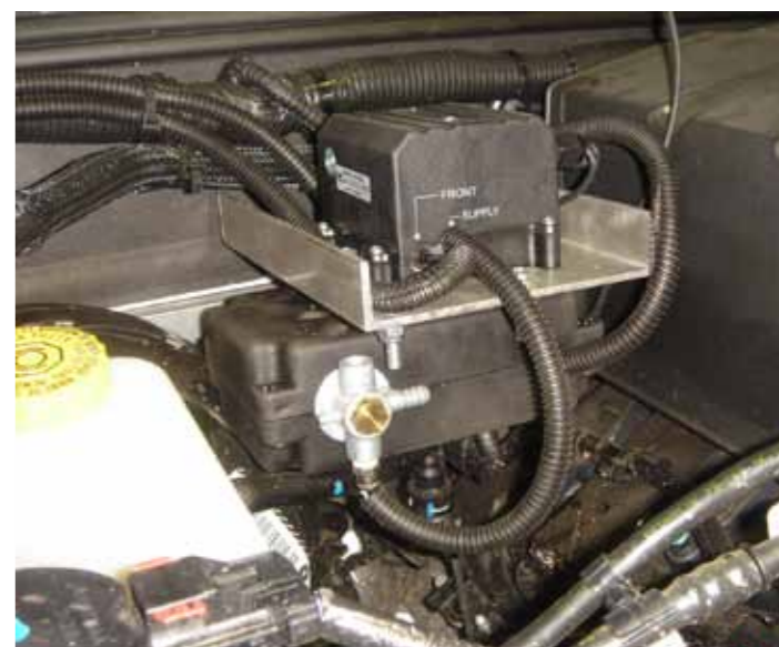
JK my ride pump install. There isn't a lot of space under the JK hood, especially the 2012 model, to fit the My-ride pump and controller. We utilized the fire wall bracket on the driver side and wired into the fuse box. you have to have a switch able power source for the My-ride as they can ghost operate when not required if hard wired when they sense a drop in line pressures.
