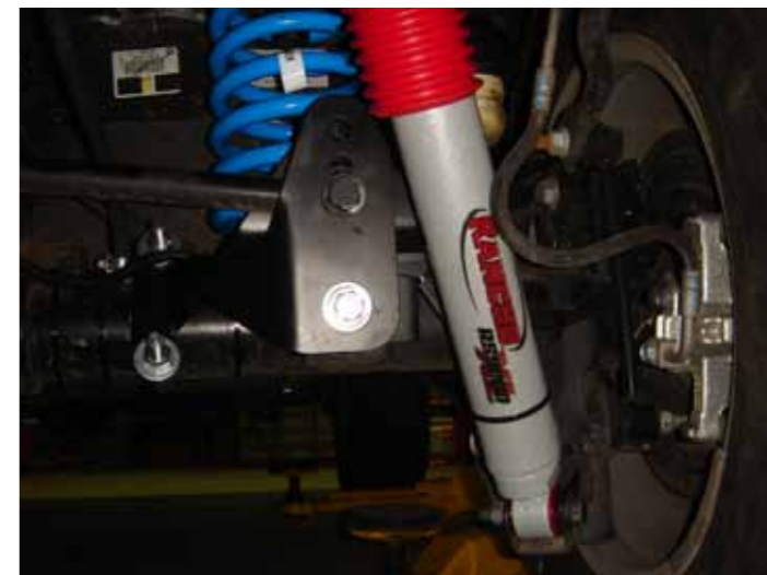
Here is the rear of the JK lift with the rancho shock, teraflex drop panard bracket and Mopar coil
