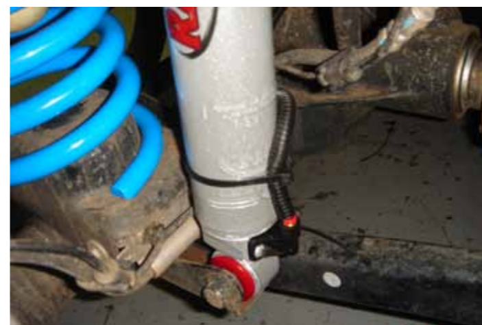
Running the air lines to the shocks needs to be carefully done so they won't foul or stretch, the fronts fitted up and extra spaghetti cover.
