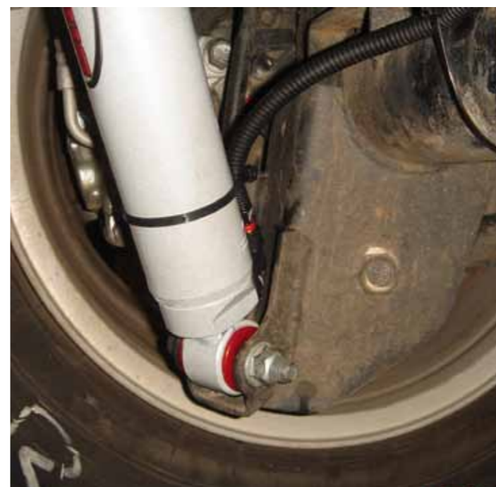
On the rear shock it's possible to run the manifold facing frontwards to protect it from damage while wheeling...this is the rear end sorted
